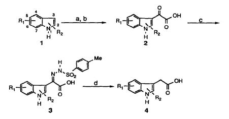
a. Oxalyl chloride, anhydrous ether, 0 °C, 20 min; b. Saturated aqueous NaHCO\_3, reflux 30 min;
